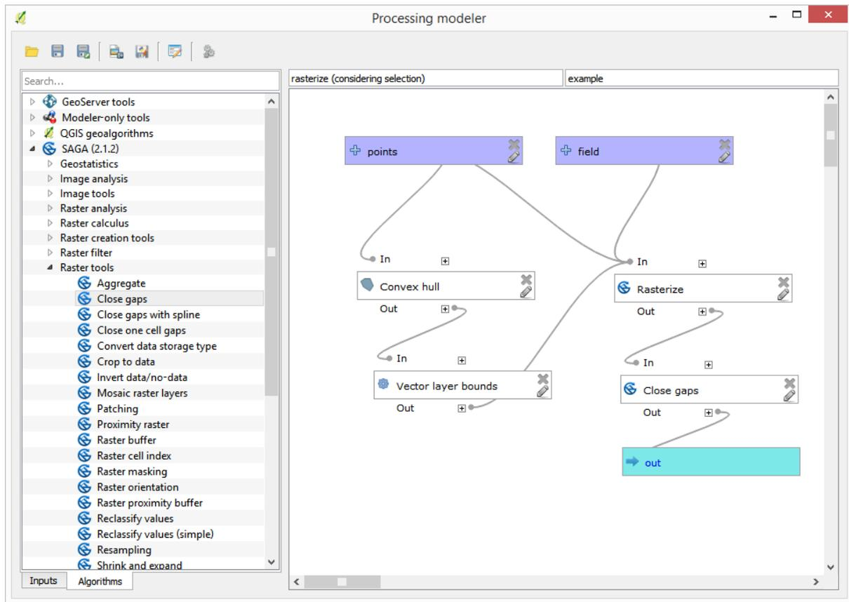
The algorithm is now ready to be saved and added to the toolbox. You can run it and it will generate a raster layer from interpolating the selected points in the input layer, and the layer will have the same extent as the selection.
