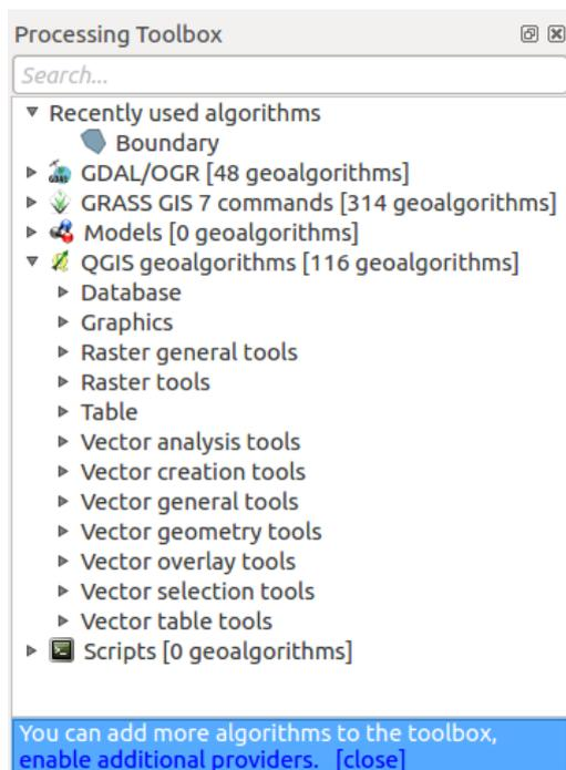
The toolbox contains a list of all the available algorithms, divided in groups so called *Providers*. Providers can be (de)activated in the settings dialog. A label in the bottom part of the toolbox will remind you of that whenever there are inactive providers. Use the link in the label to open the settings window and set up providers. We will discuss the settings dialog later in this manual.
