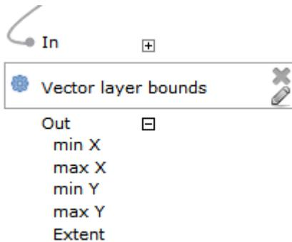
We can now add the algorithm that rasterizes the vector layer, using the extent from the *Vector layer bounds* algorithm as input.
