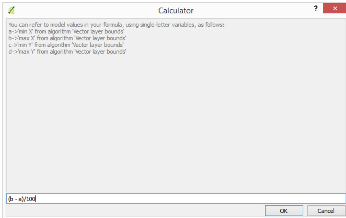
Now we have to edit the rasterize algorithm, so it uses the output of the calculator instead of the hardcoded value.
